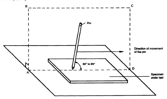
The pin is in the plane ABCD, which is perpendicular to the sample.
